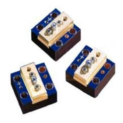
nLIGHT's industry recognized conduction cooled (CS) diode laser package features a 30% fillfactor bar that is rated at 60 W on an industry standard conduction cooled CS package. By combining nLIGHT's proprietary nXLT™ (eXtended Life Technology) laser chips with AuSn solder on an expansion-matched sub-mount, nLIGHT is able to offer a significant increase in power and brightness while increasing lifetime for CW, pulsed, and high temperature applications.
